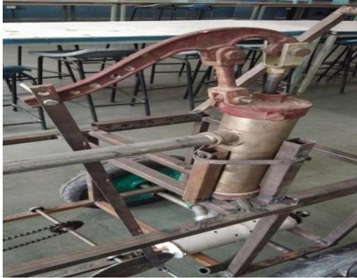
Fig. 2 Slider Crank Mechanism
