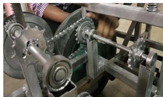
Fig. 1 Sprocket Chain Mechanism
