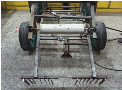
Fig.3 Weeder and Seeder Mechanism
