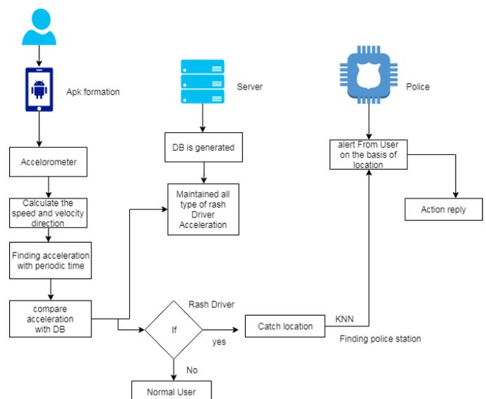
System design contains the Android application which should enable the Car Mode so that the accelerometer sensor can sense the velocity and help to detect whether the vehicle is in normal mode or rash mode. For that, ideal entries are stored in the database. Current entries will be compared with ideal database. If it is found that the
