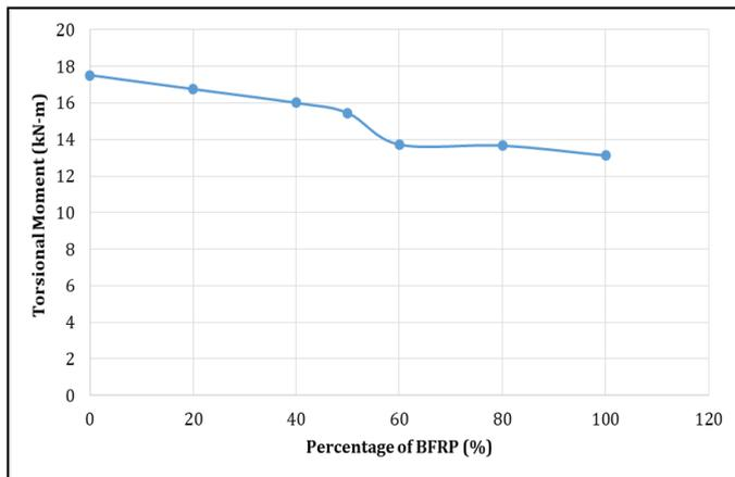
Fig -13 : Replacement of BFRP strips in between CFRP strips
