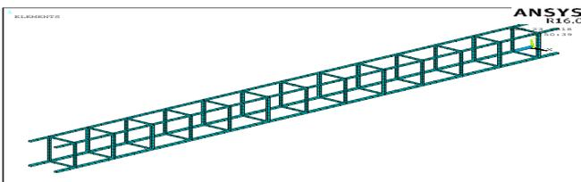
Fig -2: ANSYS Model of Control Beam
