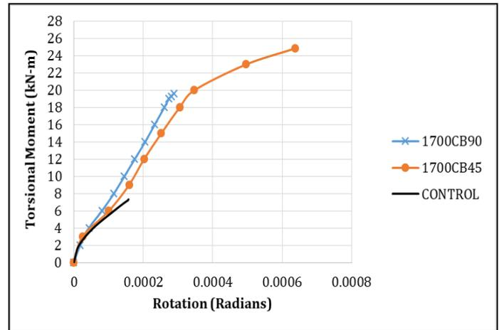
Fig -14 : Torsional Moment Vs Rotation Graph of Hybrid CFRP-BFRP (layer) Beams
