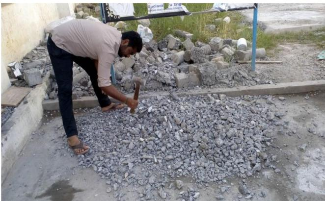
Fig -1: preparation of recycled aggregates
