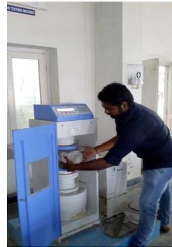
Fig. 6 split tensile strength test
