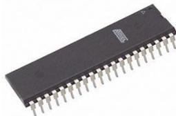
**ATmega16** is an 8-bit high performance microcontroller of Atmel's Mega AVR family with low power consumption. Atmega16 is based on enhanced RISC (Reduced Instruction Set Computing) architecture with 131 powerful instructions. Most of the instructions execute in one machine cycle. Atmega16 can work on a maximum frequency of 16MHz.
