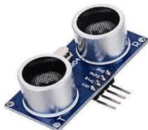
This is the HC-SR04 ultrasonic ranging sensor. This economical sensor provides 2cm to 400cm of non-contact measurement functionality with a ranging accuracy.
