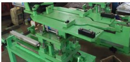
Fig -6:- Clamping and Expanding Jaws.
