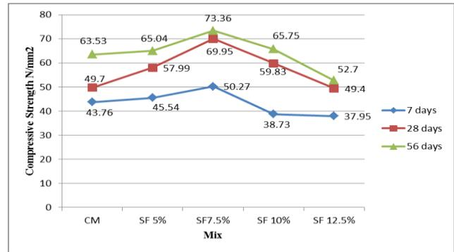
Figure 3: Compressive strength of Silica Fume variation
