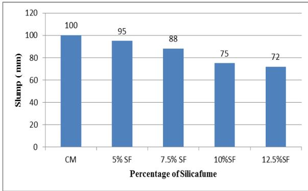
Figure 1: Slump Result of Silica Fume Variation
