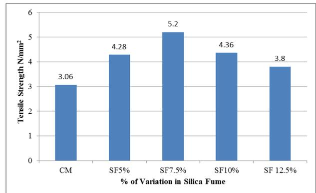
Figure 4: Effect of Silica Fume on Split Tensile Strength Concrete
