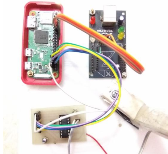
Fig 5. Transmitter Module with Raspberry PI
