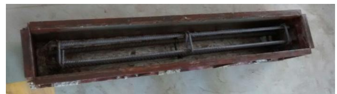
(a) Mould used for casting beams
