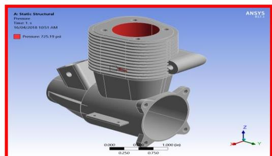
**Fig. No. 2 Pressure Applied for Engine Blower**
