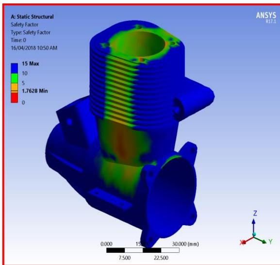
**Fig. No. 3 Safety Factor of Engine Blower**
