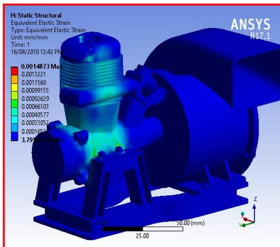
**Fig. No. 4 Equivalent Elastic Strain for Engine Blower**
