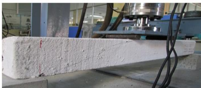
Fig 4.6 Crack pattern of 45 % of steel slag
