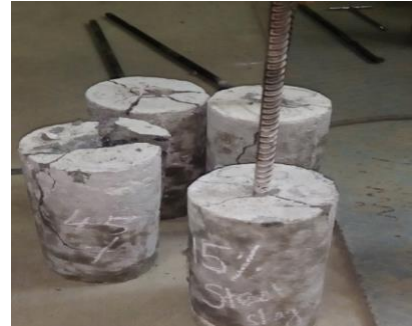
Fig 4.1 Pull out strength test specimens
