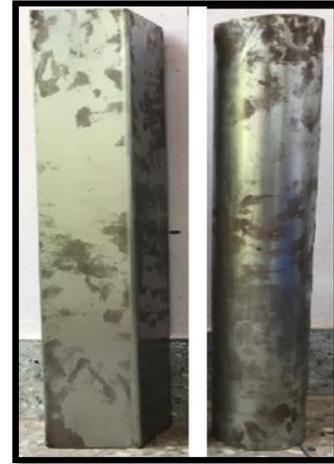
Fig -5: Concrete filled steel tubes
