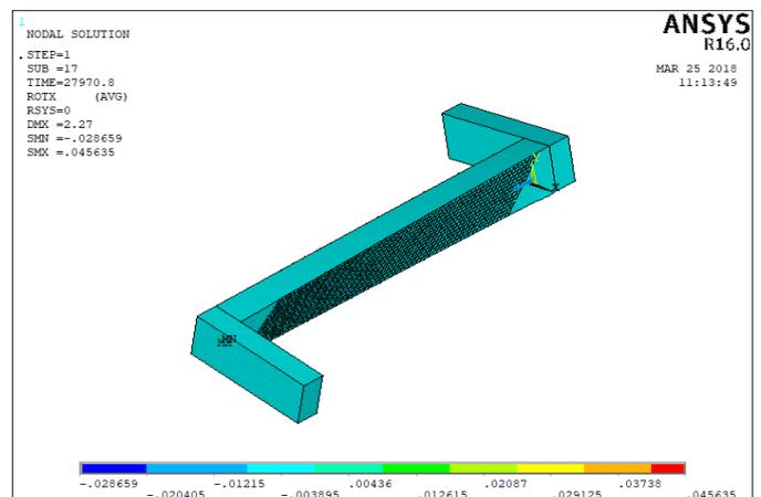
Fig -13 : Beam strengthened at 90 degree oriented sheets at failure
