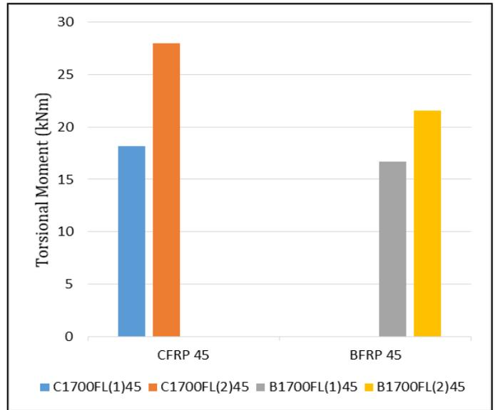
**Fig -16 :** Comparison of beams wrapped with one layer and two layer of CFRP/BFRP oriented at 45 degrees
