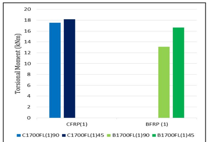
**Fig -17 :** Comparison of beams wrapped with one layer of CFRP/BFRP oriented at 90 degrees and 45 degrees
