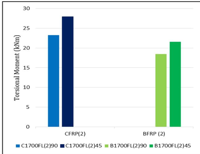
**Fig -18 :** Comparison of beams wrapped with two layer of CFRP/BFRP oriented at 90 degrees and 45 degrees
