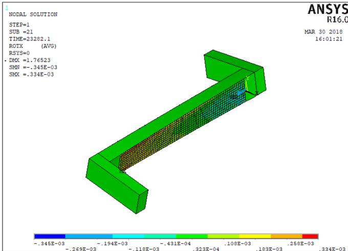
**Fig -14 :** Beam strengthened at 90 degree oriented sheets at failure
