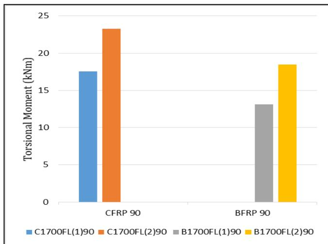
**Fig -15 :** Comparison of beams wrapped with one layer and two layer of CFRP/BFRP oriented at 90 degrees
