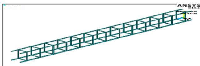
Fig -1: ANSYS Model of Reinforcement
