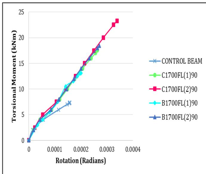
Fig -11: Torsional Moment Vs Rotation Graph of Beams with 90 Degree Oriented Wraps
