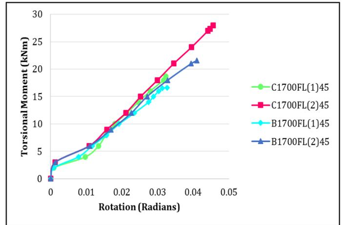
Fig -12: Torsional Moment Vs Rotation Graph of Beams with 45 Degree Oriented Wraps
