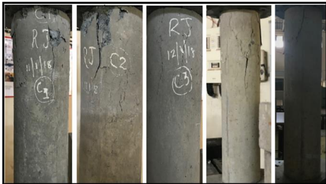
Fig -2: Crack pattern PCS circular specimens
