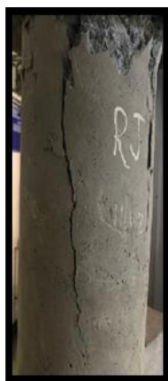
Fig -3: Crack pattern for rebar specimen
