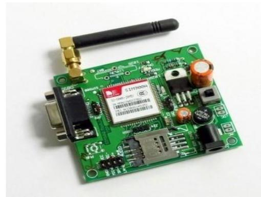
Figure- 2: GSM Module
