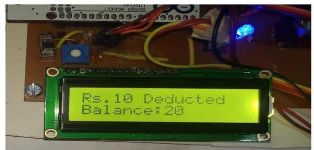
Figure- 7: LCD Display Showing the balance if a person enters the parking slot
