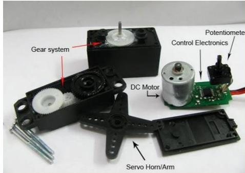
Figure -3: Servomotor
