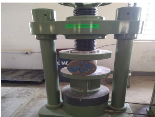
Fig -6: split tensile strength test set-up
