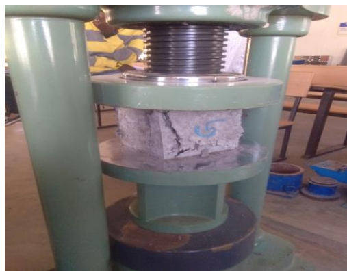
Fig -4: Compressive strength test set-up
