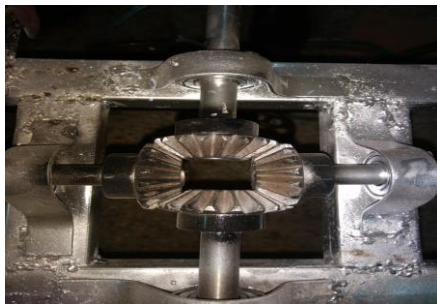
Arrangement of gear for power transmission
