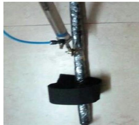
Fig-2: Fabricated right shoulder pneumatic cylinder
