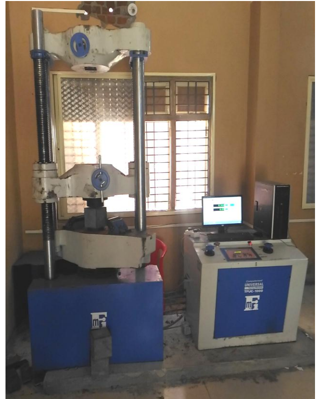
Fig - 2 : UTM Machine Setup
