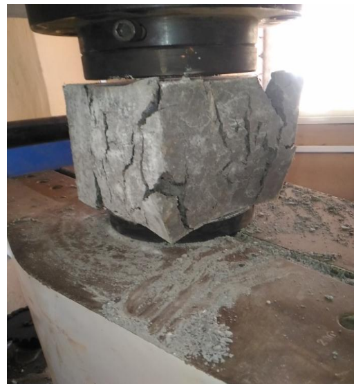
Fig - 3 : Failure of Concrete Cube
