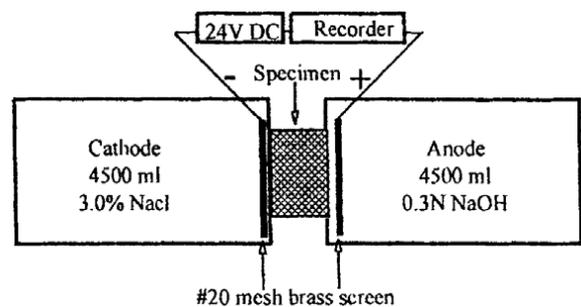
Fig -5.1.1 Schematic diagram of ACMT cell
