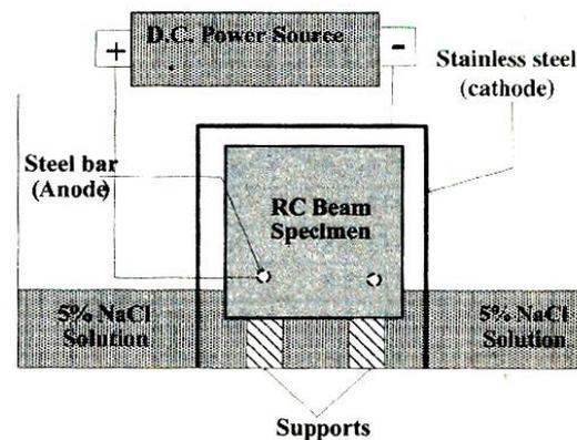
Fig -3.2: The set-up used by Azad et al. for accelerating reinforcement corrosion
