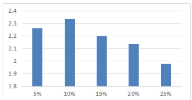
**Graph 3: Split tensile Strength replacement of fly Ash**
