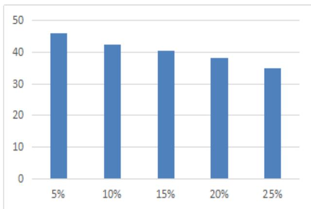
**Graph 1: Compression strength with replacement of fly Ash**
