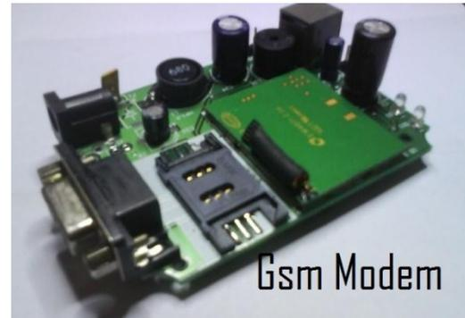
Fig.2 GSM Modem
