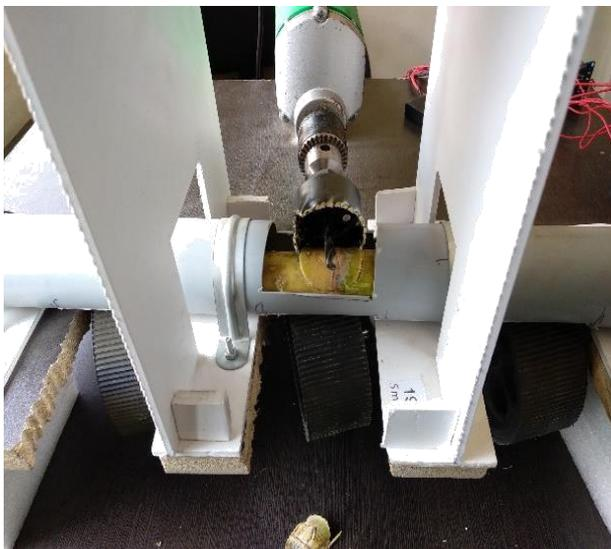
Fig -5.3: Cutting Process of Sugarcane.
