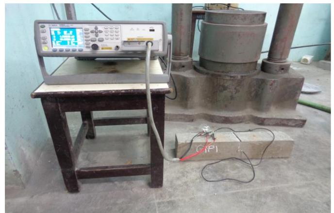
Fig. 3 Experimental setup of signature acquisition.
