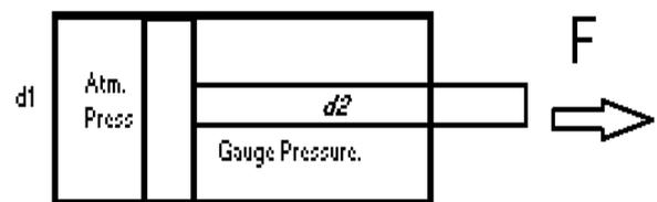
Fig -1: Double Acting Cylinder
