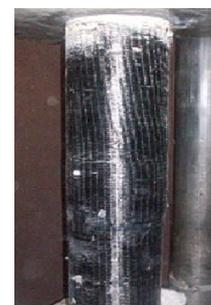
**Fig-5:** Behavior of Four layered CFRP Wrapped column in Transverse orientation under Axial load
