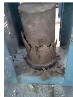
Fig-2: Compressive strength of concrete
