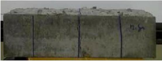
**Fig-6: Prism Test**
