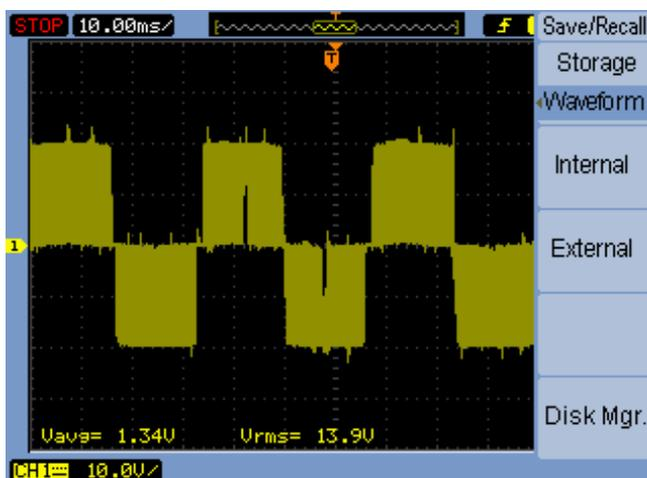
Fig 9: Inverter output pulse
