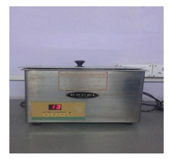
Figure 3.5 Preparation of .5 wt. % Al<sub>2</sub>O<sub>3</sub> Nanofuel
