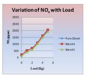
Figure 4.9 Variation of NOx with Load
