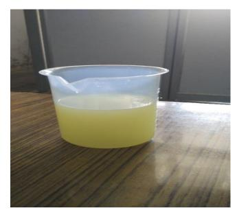
Figure 3.6 Prepared Al<sub>2</sub>O<sub>3</sub> blended Nanofuel
