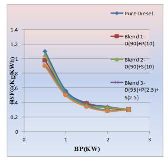
Figure 4.3 Variation of brake specific fuel consumption with brake power
