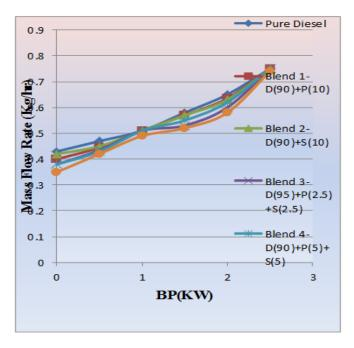
4.1.1 Variation of mass flow rate of fuel with brake power
