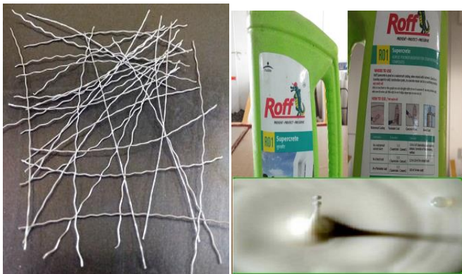
Fig. 3 Steel fiber and Acrylic polymer
