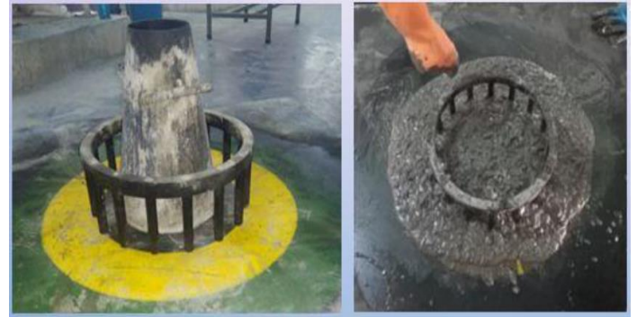
Fig -4: J- Ring Test (a) Setup (b) After releasing possibility checking
