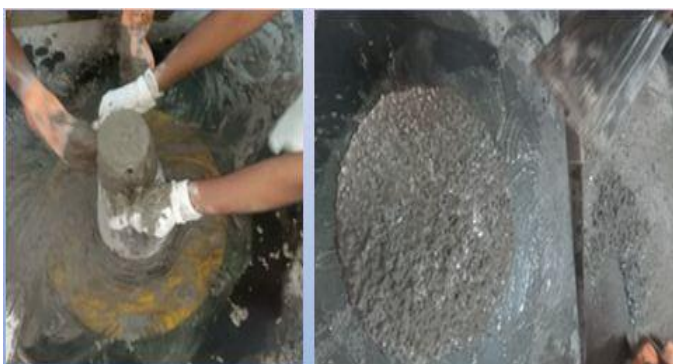
Fig -3: Slump flow test (a) Before releasing cone (b) After releasing the cone
