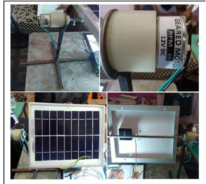
Fig 8. Portable Solar Tracking System
