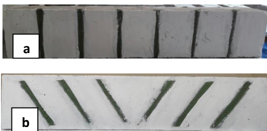
Fig -5: Strengthened beams; a.NB-8d-90 and b.NB-8d-45
