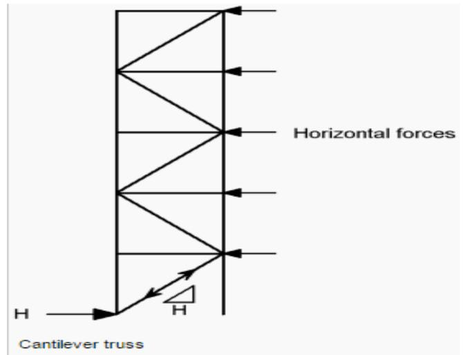
Fig-2: Vertical Bracing System
