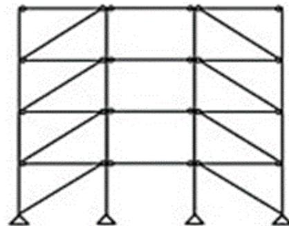
Fig-4: Single Bracing
