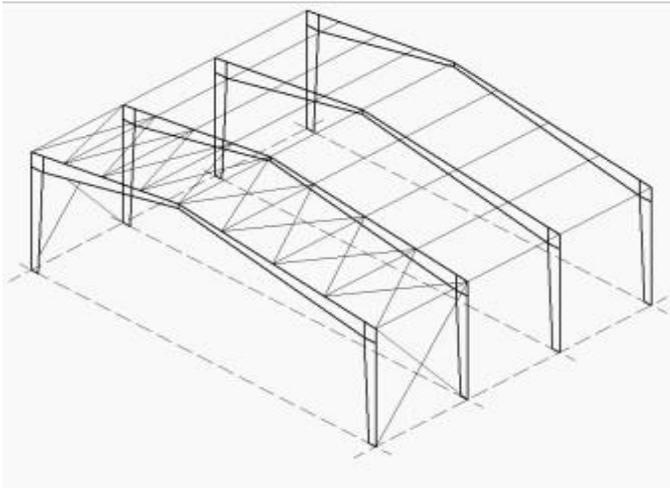
Fig-3: Horizontal Bracing System
