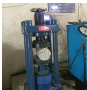
Fig-10: Split tensile Strength Testing
