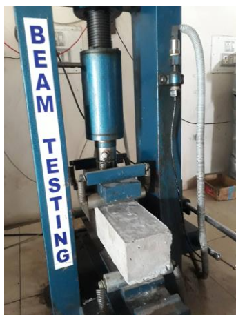
Fig-9: Flexural Strength Testing
