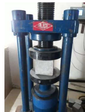
Fig-8: Compression Strength Testing
