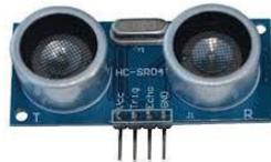
Fig - 4 :Ultrasonic sensor Pin diagram [9]
