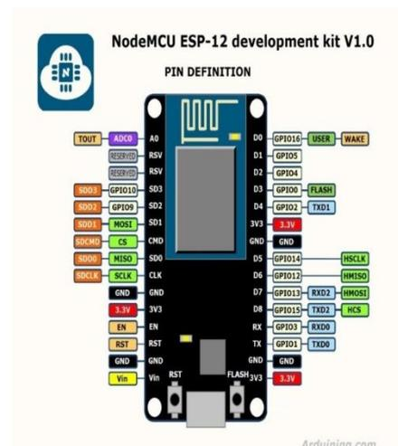
Fig- 3 :Pin diagram of NodeMcu[9]
