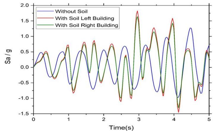
Figure-8: Acceleration response for group of two identical buildings (Fixed base and with SSI).
