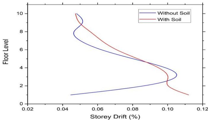
Figure-6: Storey Drift for Single Building (Fixed base and With SSI).
