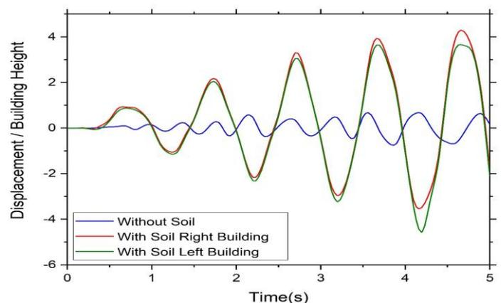
Figure-9: Displacement for group of two identical buildings (Fixed base & with SSI).
