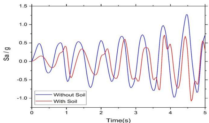
Figure-4: Acceleration response for single building (Fixed base and With SSI).
