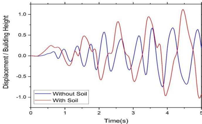
Figure-5: Displacement for single building (Fixed base & with SSI).
