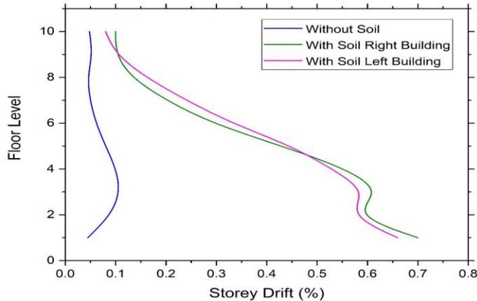
**Figure-10:** Storey Drift for group of two identical buildings (Fixed base & With SSI).
