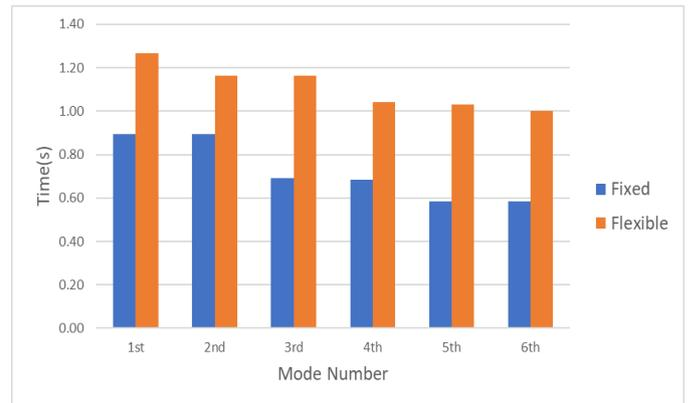
Figure-7: Variation in time period for group of two buildings (Fixed base & with SSI).
