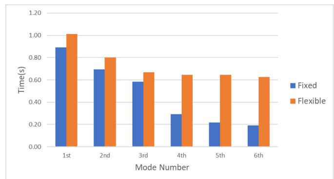
Figure-3: Variation in time period for single building (Fixed base and with SSI).
