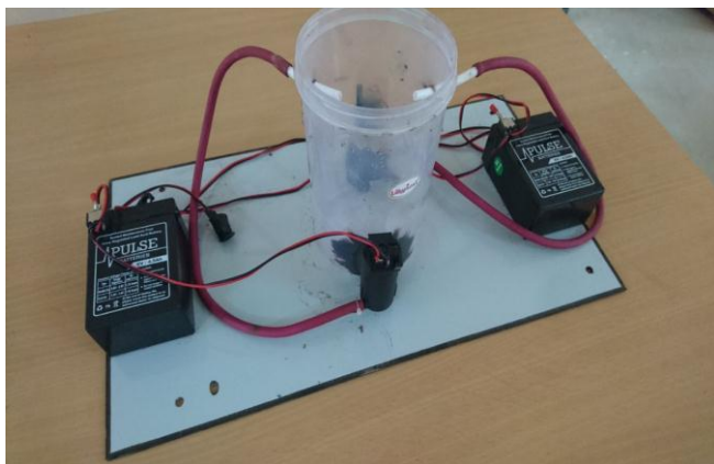
Fig. 7: Pump assembly, Reservoir and Battery
