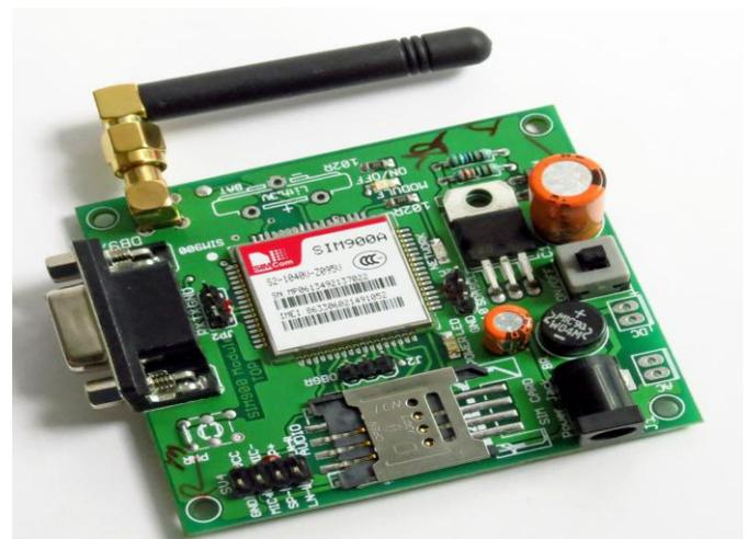
Fig -2: GSM Transceiver SIM900
