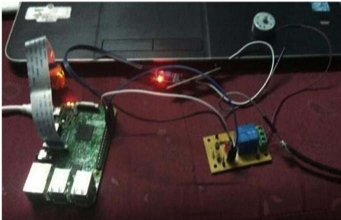
**Fig -2:** Proposed system with soil moisture and water pump for the irrigation system.
