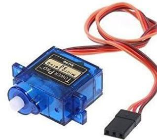
Fig 3: Servo Motor
