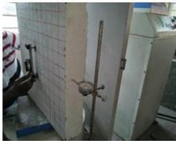
c. Strain gauge and dial gauge attachment
