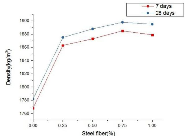
Figure7: Densities at different percentage of Steel fibers
