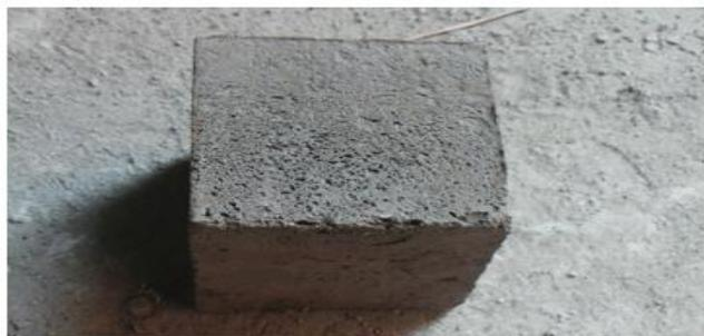
**Figure 2:** Lightweight concrete cubes
