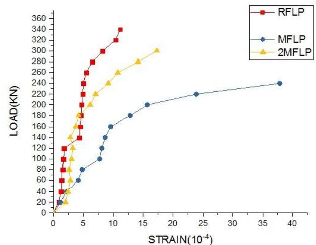
Figure 12: Strain variation across the mid-height FLC of panels at different load stages.
