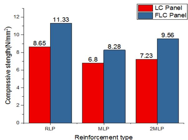
Figure 9: Compressive strength of panels at different reinforcement cases
