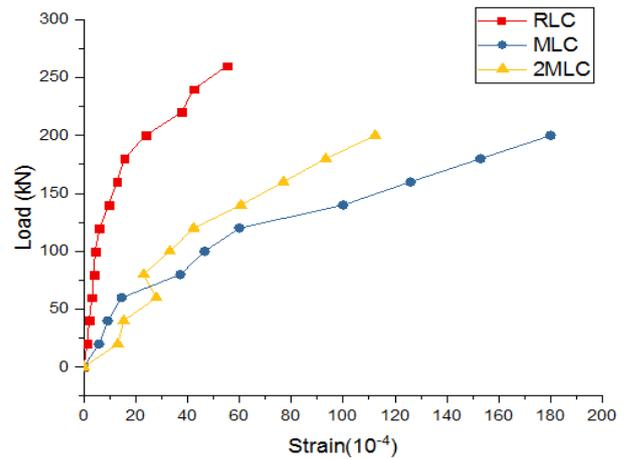
Figure 11: Strain variation across the mid-height of LC panels at different load stages.
