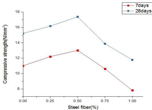
Figure 8: Compressive strength at different percentage of steel fibers
