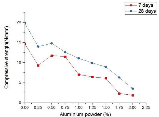
Figure 6: Compressive strength at different percentage of aluminium powder for 1:2 mix
