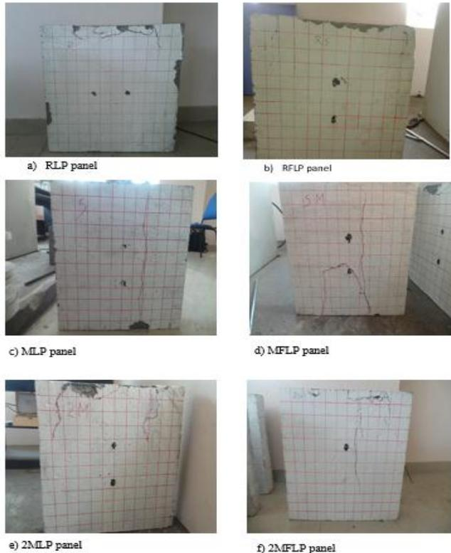
Figure 10: Failure pattern of lightweight concrete wall panels
