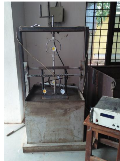
Fig 1 : Model test tank and loading arrangement
