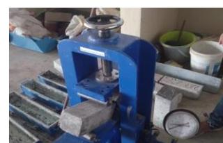
**Fig-2:** Testing for flexure strength
