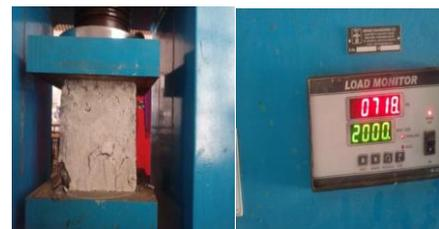
**Fig:** compressive strength testing of cube
