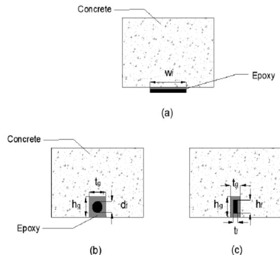
Fig -1: FRP strengthening methods (a) EBR FRP plate or sheet (b) NSM FRP rod or bar (c) NSM FRP laminate or strip.
