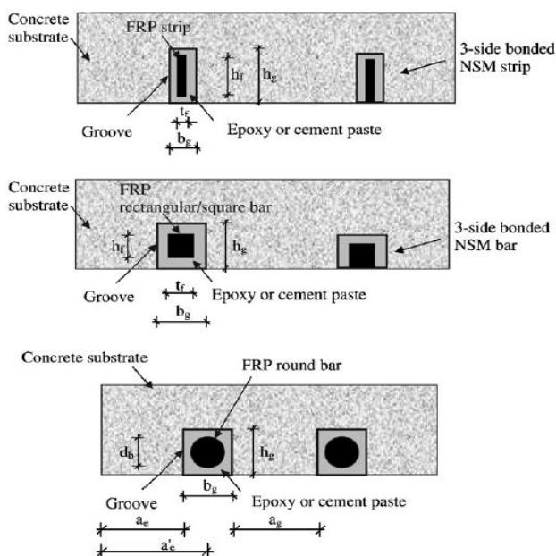
**Fig- 4. Configurations of NSM FRP reinforcement**
