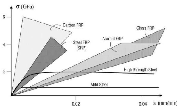
Fig-2: Strength characteristics of different fibres
