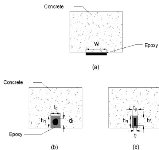
Fig -1: FRP strengthening methods (a) EBR FRP plate or sheet (b) NSM FRP rod or bar (c) NSM FRP laminate or strip.
