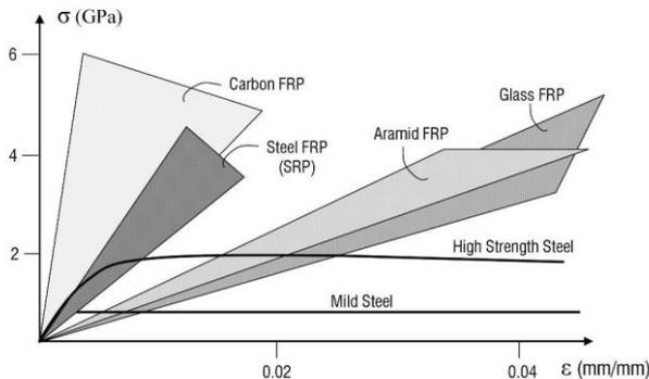
Fig -2: Strength characteristics of different fibres
