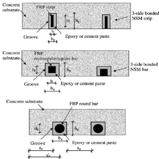
Fig- 4. Configurations of NSM FRP reinforcement
