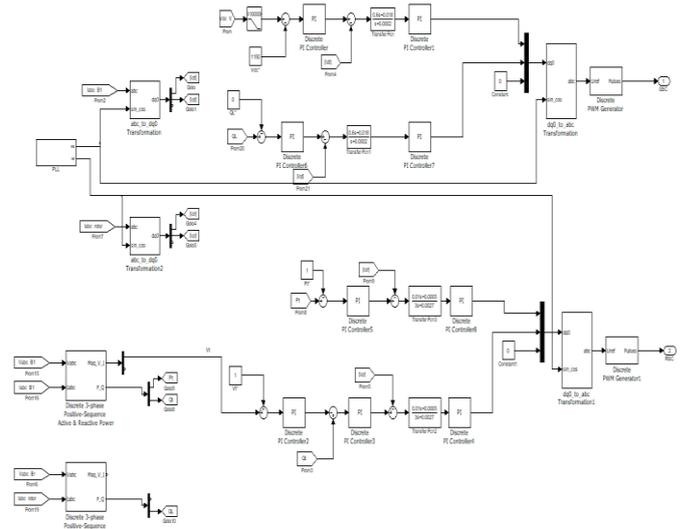
Figure 10. Controller of DFIG wind farm
