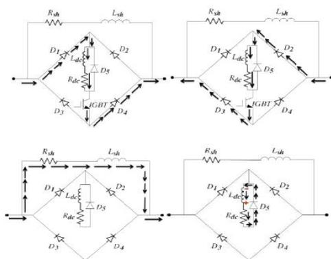
Figure: 5. Bridge Type Fault Current Limiter Operation
