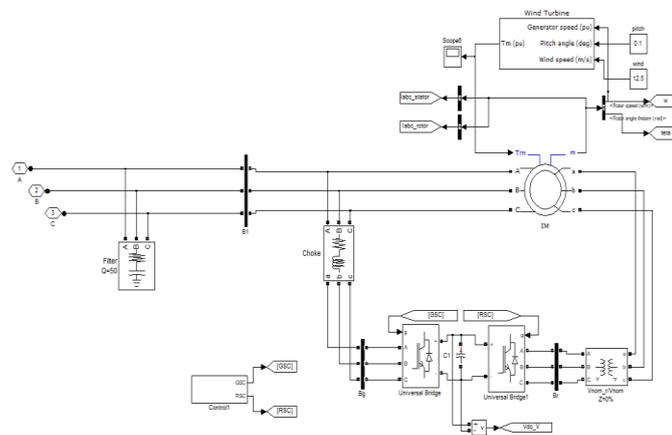
Figure 9. DFIG modeling for 2MW wind farm
