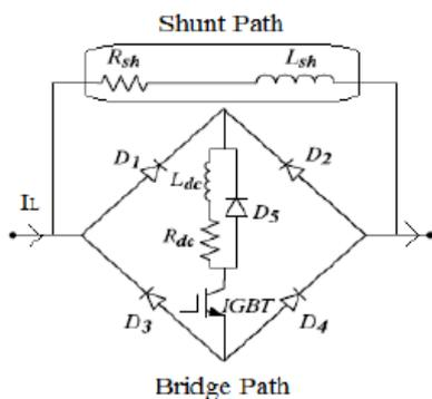
Figure: 4. Bridge Type Fault Current Limiter
