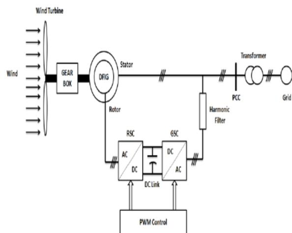
Figure: 1. Basic diagram of DFIG wind turbine
