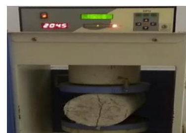
Fig- 5: Split tensile strength test
