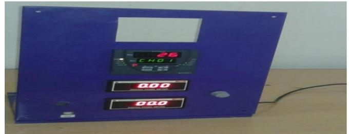
Fig.3 Photograph of Data logger
