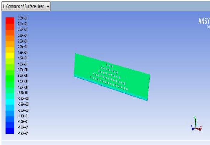
Fig. 9. Contours Of HTC Of Variable Porous Pin Fin
