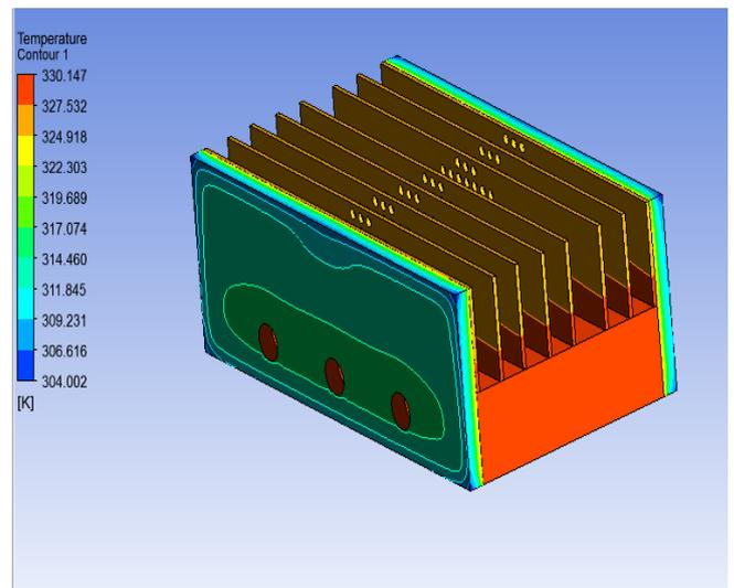
Fig 6 Contours Of Temperature Of Full Assembly
