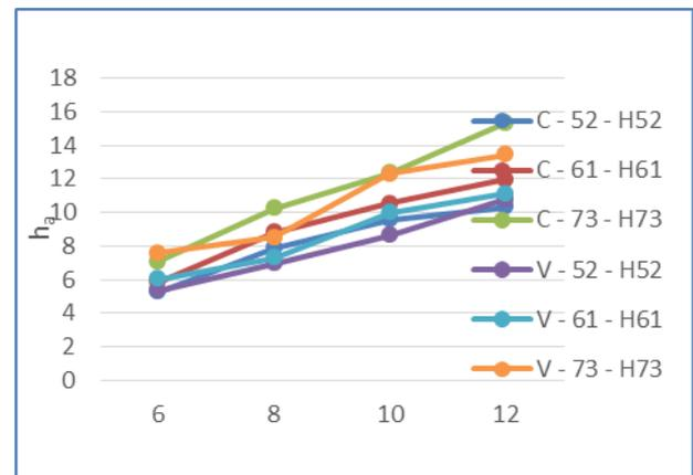
Chart.1. Variation of  $h_a$  W.R.T Spacing between fin plates for constant pitch 30° perforation and 4 mm perforation diameter.
