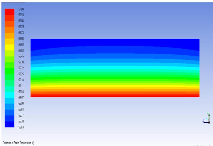
Fig.10 Contours of Static Temp of Plane Pin Fin
