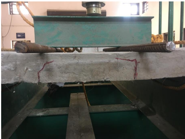
Fig -2Crack on panel after loading
