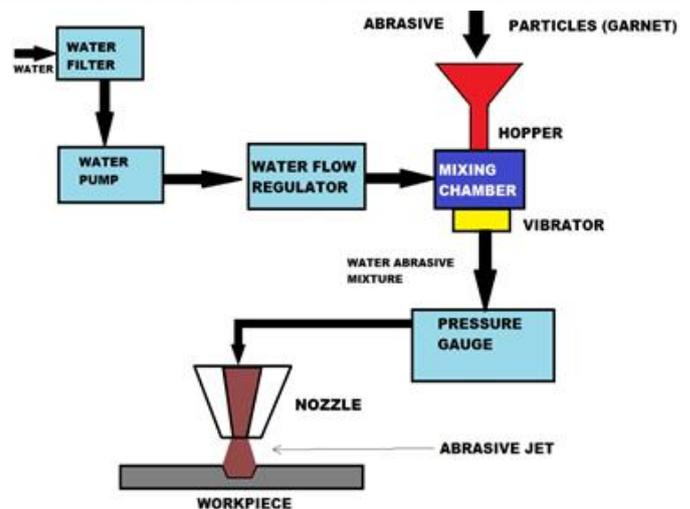
Fig -1: Abrasive Water jet machining.
