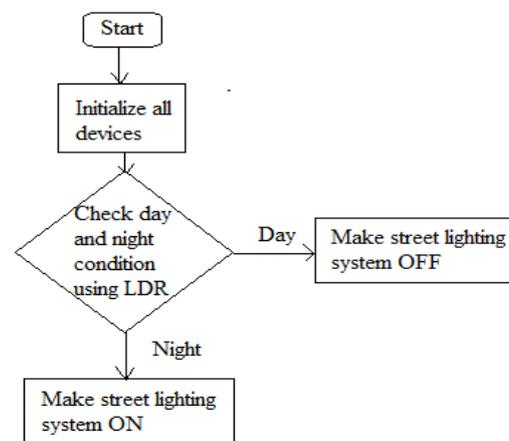
Fig -2: Flowchart for checking day and night condition using LDR
