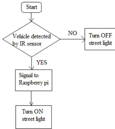
Fig -3: Flowchart for vehicle detection
