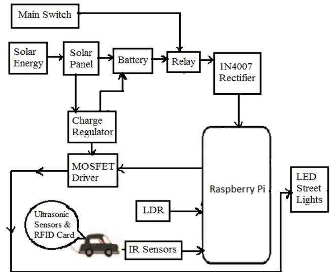
Fig -1: Block Diagram of Vehicle Movement using Street Light Detection
